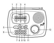
1. **LCD Display** Displays time, channel, frequency, and functions.
